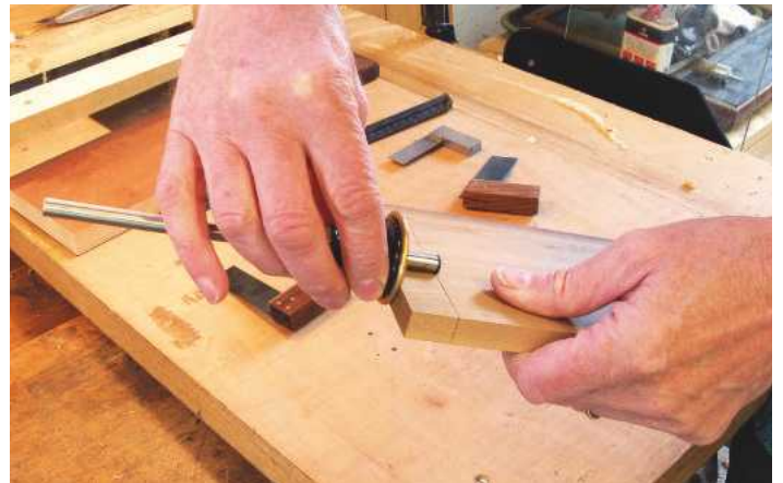
▲ Pic.3 Marking thickness of pin board on tail board
